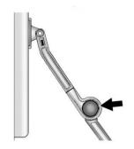
Press the red button on the prop rod to close the cover.
